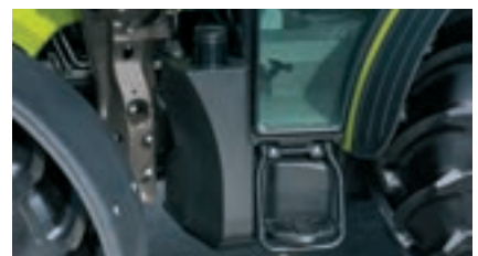
Refuelling the ELIOS is straightforward as the filler neck is conveniently located to the left of the cab access steps.
