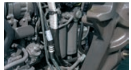
The oil filters in the engine are easy to reach even with a front loader bracket.
