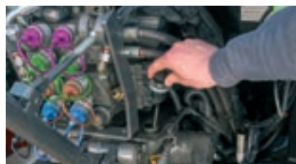
The transmission and hydraulic oil level is checked at the rear using a dipstick.
