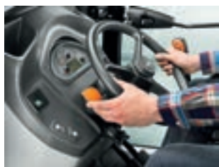
The reverser for mechanical reversing and the electronic REVERSHIFT is handily positioned to the left of the steering wheel.
