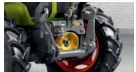
The optional front linkage with 2.8 t lift capacity extends the range of ELIOS applications.
