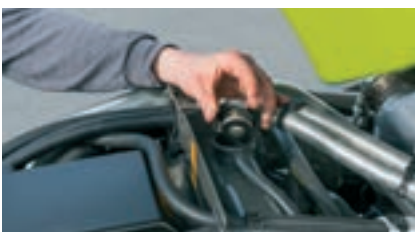
The coolant level can be checked at the radiator expansion tank.
