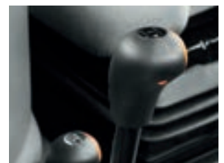
With REVERSHIFT: the electronic clutch is operated by pressing a button on the gear lever.
