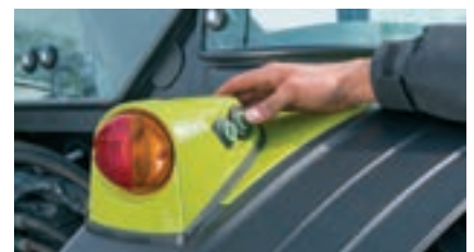
For implement attachment, the electronic and mechanical rear linkage can be operated externally at the rear of the tractor.
