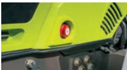
The battery isolating switch is built into the bonnet for ease of access.
