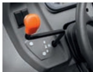
The reverser for mechanical reversing and the electronic REVERSHIFT is handily positioned to the left of the steering wheel.
