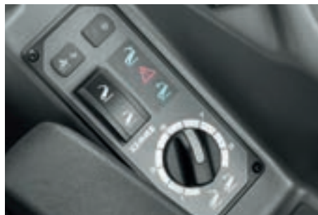
Control panel for the electronic rear linkage: quick-lift, lower and quick-entry. The dial is used to pre-set the working depth.
